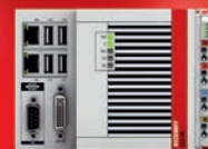
CX5140: Intel®-Atom™-CPU, 1,91 GHz, quad-core
