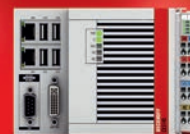
CX5140: Intel®-Atom™-CPU, 1,91 GHz, quad-core
