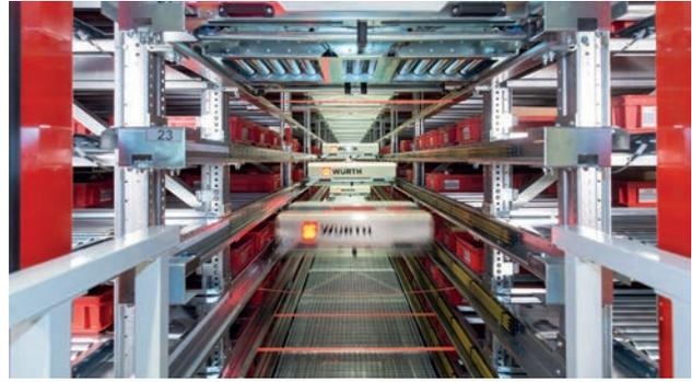
Highest storage capacity and flexibility with the OSR Shuttle™
